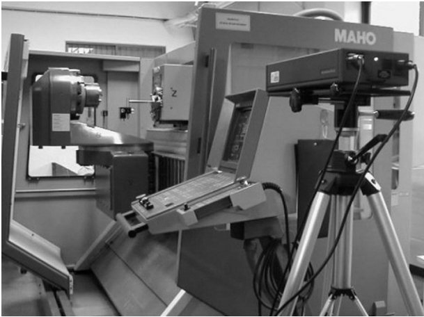
Fig. 7. Direct measurement with interferometer.
