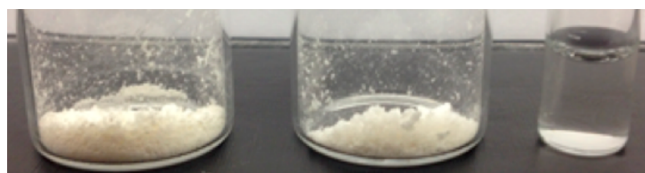
Figure 6. From left to right: photographs of lidocaine hydrochloride (5-HCl) obtained after reactive crystallization (purity 94%, HPLC); 5-HCl obtained after antisolvent cooling crystallization (purity 97.7%, HPLC), and formulated 5-HCl (20 mg mL -1 ).
