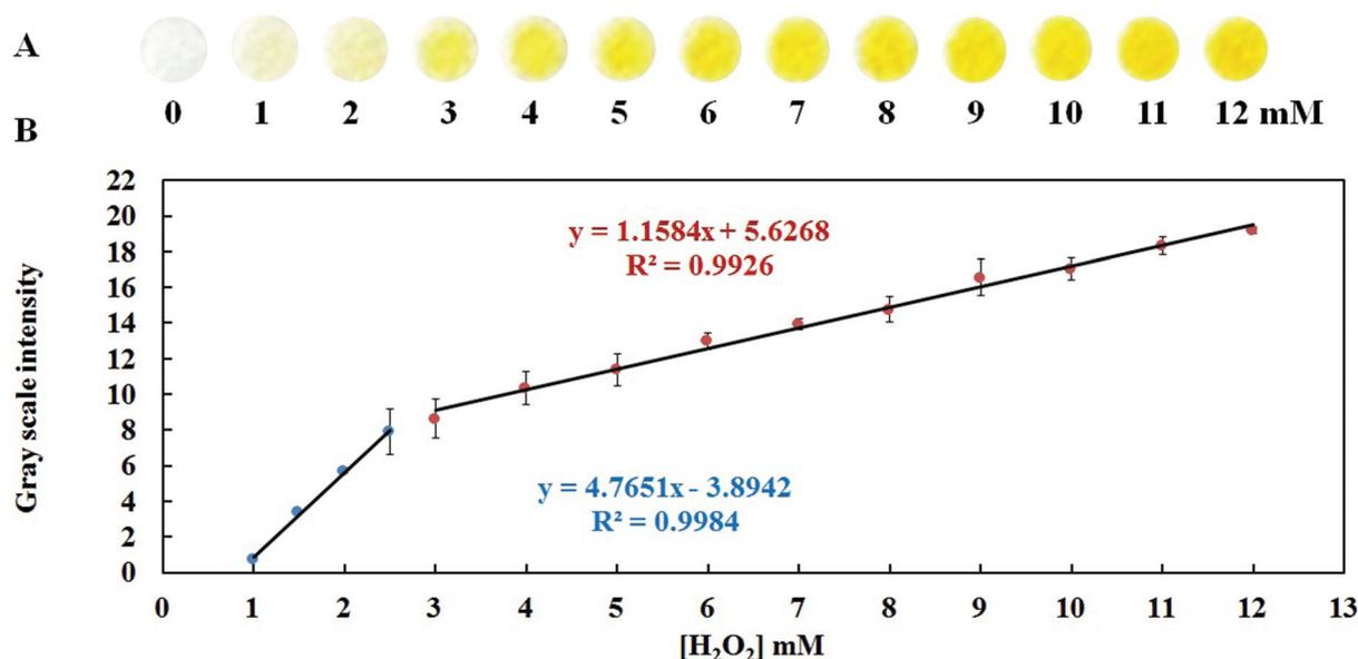
Fig. 1 The analysis of H<sub>2</sub>O<sub>2</sub> using nanoceria-coated paper-based devices. (A) Typical devices from the analysis of different concentrations of H<sub>2</sub>O<sub>2</sub>. (B) Standard curve plotted of gray intensity as a function of H<sub>2</sub>O<sub>2</sub> ( $n = 3$ ) giving two linear portions where the first one has higher sensitivity than the second portion as the intensity became saturated at higher H<sub>2</sub>O<sub>2</sub> concentrations.
