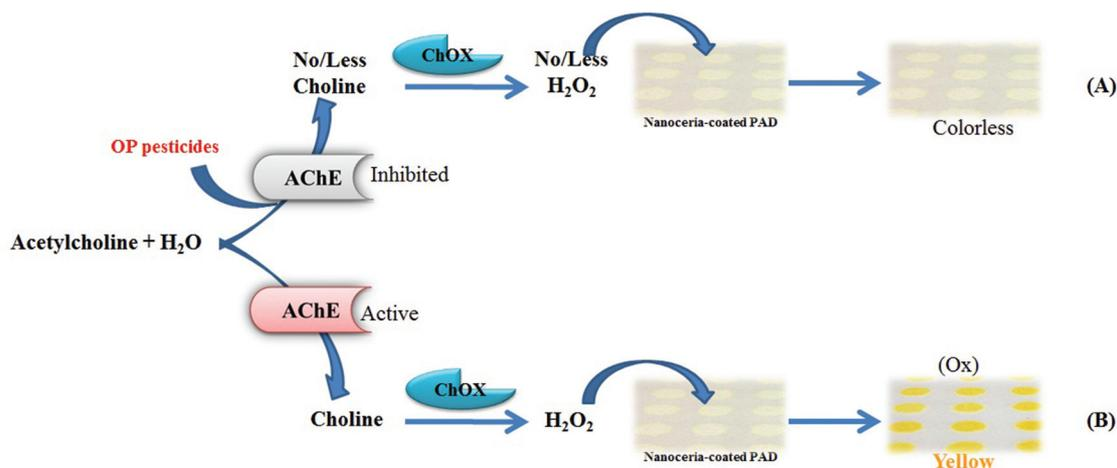
**Scheme 1** Paper-based device for the analysis of OP pesticides using enzymatic assay and nanoceria as colorimetric agents. (A) Upon the addition of OP pesticides, AChE activity is inhibited resulting in no/less H<sub>2</sub>O<sub>2</sub> and hence less nanoceria color developed. (B) Without the addition of OP pesticides, AChE activity is normally active producing H<sub>2</sub>O<sub>2</sub> that causes the color change of nanoceria.
